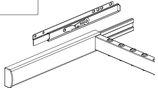
Step 3: Screw inner channel to aluminum spacer. Join outer slide together with the inner channel.
