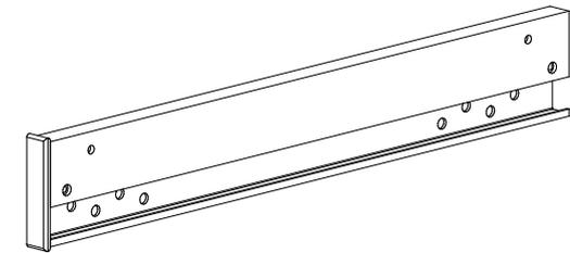
Step 2: Push part "D" to get the inner channel out.
